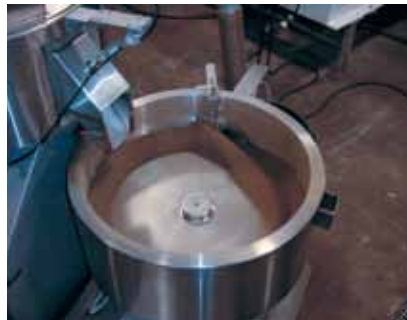
Agglomerations are sized and shaped utilizing a high speed centrifugal process.
